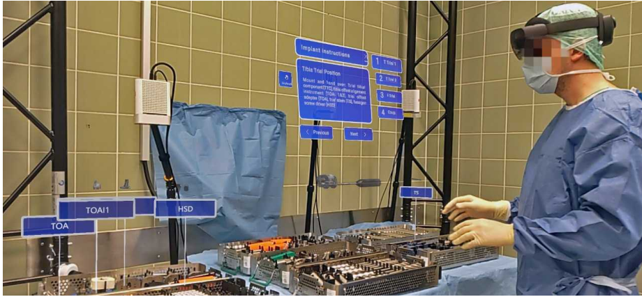
Fig. 1: Informed by marker-free multi-camera pose estimation, our AR guidance system visualizes tooltips and an assembly animation for knee arthroplasty.
